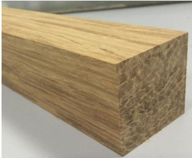
Bamboo scrimber/ Parallel bamboo strand lumber (PBSL)
